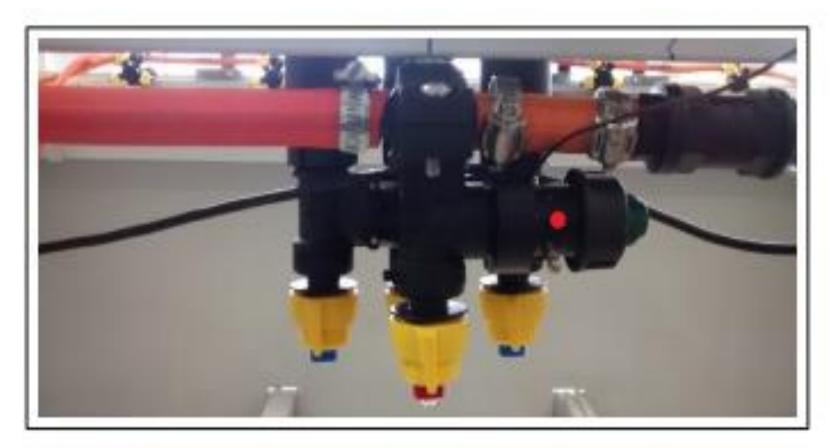
Instrumental arrangement for validation of the intelligent sensor to measure response time of a direct injection sprayer with TeeJet® QJS Multiple Nozzle Bodies e-ChemSaver.
