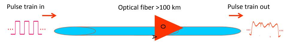
To combat with dispersion, we use optical dispersion-compensating modules, DCM (shown) and dispersion-management techniques to compensate for both chromatic dispersion, CD, and polarization-mode dispersion, PMD. However, over the long distance the dispersion accumulates and eventually the designers had to use the electro-optical regenerators. Today we encounter new problem: Existing optical networks based on DCM and dispersion management can't support transmission at 100 Gb/s.
