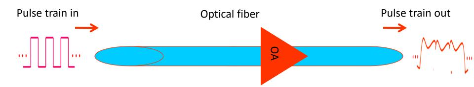
•Problem: We must limit the maximum transmission power , P, to minimize nonlinear phenomena, which results in restriction of transmission distance and also restricts the possibility to directly improve OSNR by increasing the signal power. •Refractive index of optical fiber consists of linear and nonlinear parts with respect to E' that is,  $n(\omega, E) = n_1(\omega) + n_2E^2$ .
