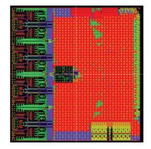
CMOS receiver ASIC with four 23 Gsample/s ADCs and DSP executing 12 trillion (12x10<sup>12</sup>) operations per second.
