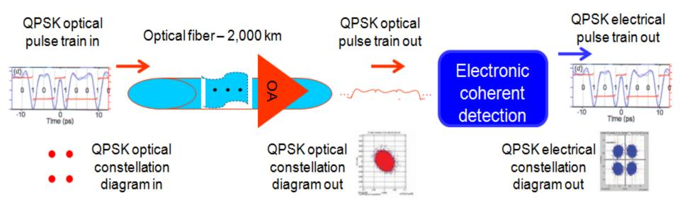
Coherent transmission replaces an optical DCM in the link with DSP electronics in the receiver, thus providing dispersion compensation in electronic domain. Though optical amplification is still necessary, the transmission distance has increased thanks to coherent detection.
